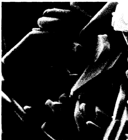
Fig. 2. Typical grain shapes of \text{MoO}_3 as observed with scanning electron microscopy (20,000 \times ).
